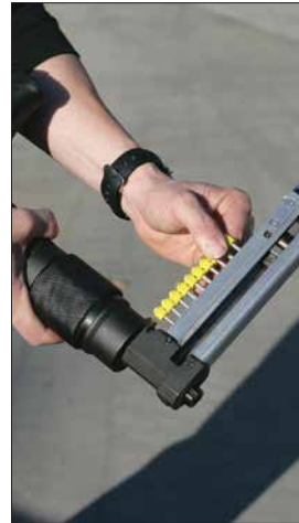
Collated pins make for fully automatic fastening and quick loading.
