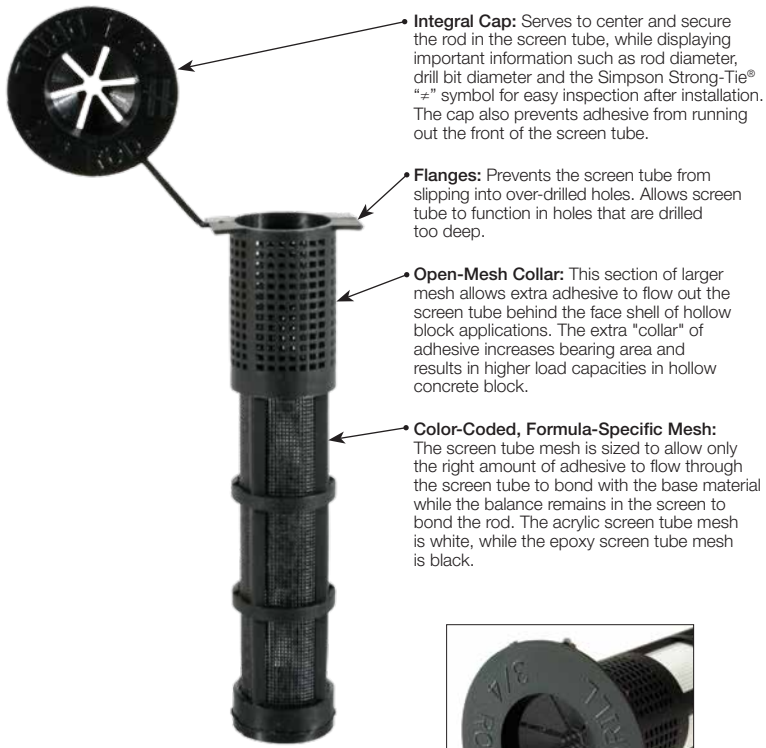
Epoxy Adhesive Screen Tube (mesh is black)
